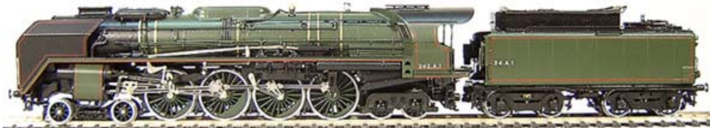
French Super Power: This was the one and only French 4-8-4, the SNCF 242A1 Type of 1948, designed by French steam locomotive genius Andre Chapelon. Dynamometer comparisons with the NYC Niagara showed the French locomotive coming out on top (hp per pound of weight). Only one 242A1 was built, and it performed well. But its complex inside running gear (this was a 3-cylinder compound) proved its undoing. it was very difficult to service, and this finally led to its being placed in storage! It is now in the French Railway Museum at Mulhouse. The photo is of an O-gauge model by Fulgurex.
